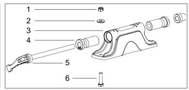
Mount the Bike Carrier to rigid surface. Losen each end of the Skewer to a width that will accommodate the forks. Remove the front wheel of the bike. Place the forks over the Skewer shaft.
